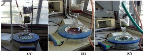
Photo plate No. 3: Extraction by soxhlet apparatus (A) Extraction of stem, (B) Extraction of flower, (C) Extraction of leaf
